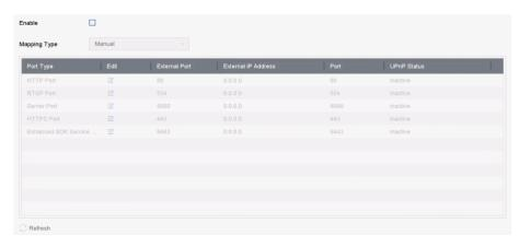
Figure 12-4 Port Mapping Setting
