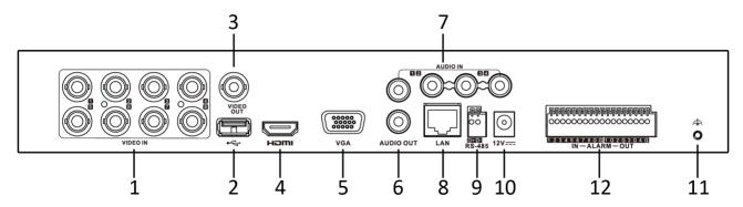
Figure 1-18 Rear Panel of iDS-7200HUHI-K1/4S(B)
