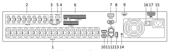
Figure 1-29 Rear Panel of DS-8100HQHI/HUHI-K8 (with 32-ch Video Inputs)
