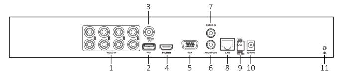
Figure 1-21 Rear Panel of iDS-7200HUHI-M2/S
