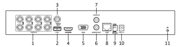
Figure 1-20 Rear Panel of iDS-7200HUHI-M1/S
