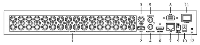
Figure 1-33 Rear Panel of DS-7200HGHI-K2
