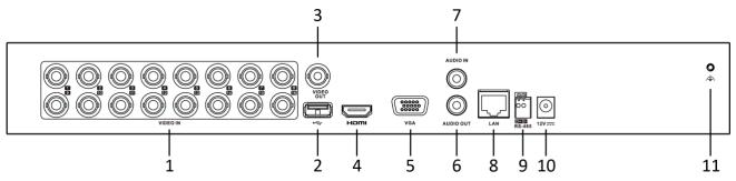
Figure 1-16 Rear Panel of iDS-7200HQHI-K2/S(B) and iDS-7200HQHI-M2/S (with 16 Video Inputs)
