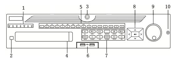
Figure 1-4 Front Panel of DS-9000HUHI/HTHI-K8 and iDS-9016HUHI-K8/16S
