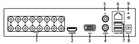
Figure 1-32 Rear Panel of DS-7200HGHI-K1
