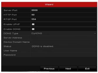
Figure 2-19 Advanced Network Parameters
