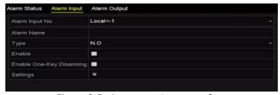
Figure 8-5 Alarm Input Setup Interface
