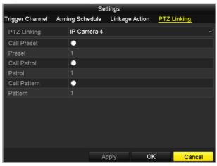
Figure 8-7 Set PTZ Linking of Alarm Input
