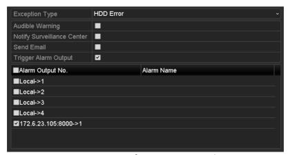
Figure 14-29 Configure HDD Error Alarm
