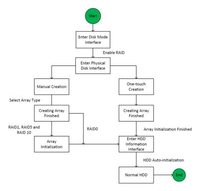
Figure 13-1 RAID Working Flow
