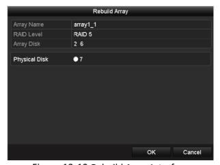
Figure 13-12 Rebuild Array Interface
