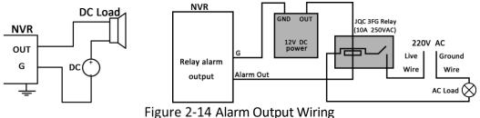
Figure 2-14 Alarm Output Wiring
