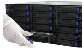
Figure 2-8 Pull out Slot
