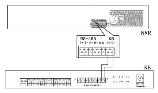
Figure 2-15 Controller Connection
