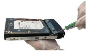
Figure 2-9 Fix the Hard Disk
