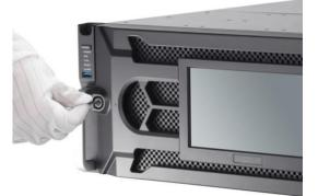
Figure 2-6 Unlock the Panel
