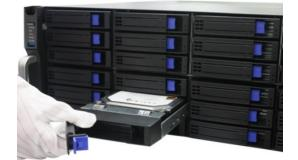
Figure 2-10 Push the Hard Disk Box into the Slot
