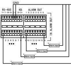
Figure 2-13 Alarm Input Wiring
