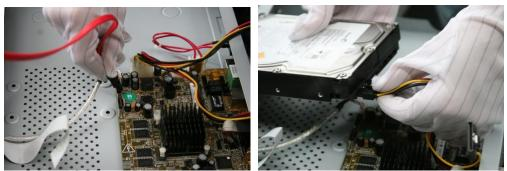
Figure 2-2 Connect Data Cable
