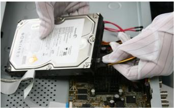
Figure 2-3 Connect Power Cable
