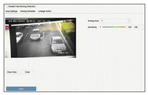
Figure 5-6 Fast moving detection
