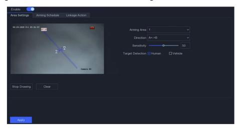
Figure 5-10 Line Crossing Detection
